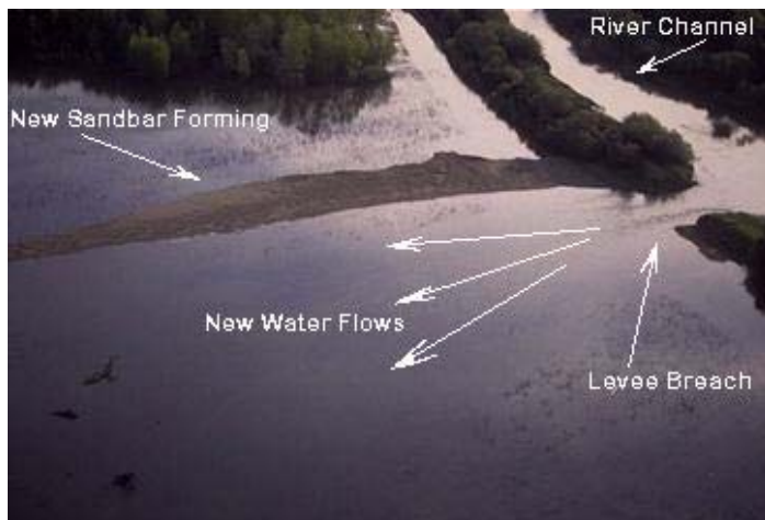
SUCCESSFUL LEVEE BREACH FOR FLOOD MANAGEMENT
